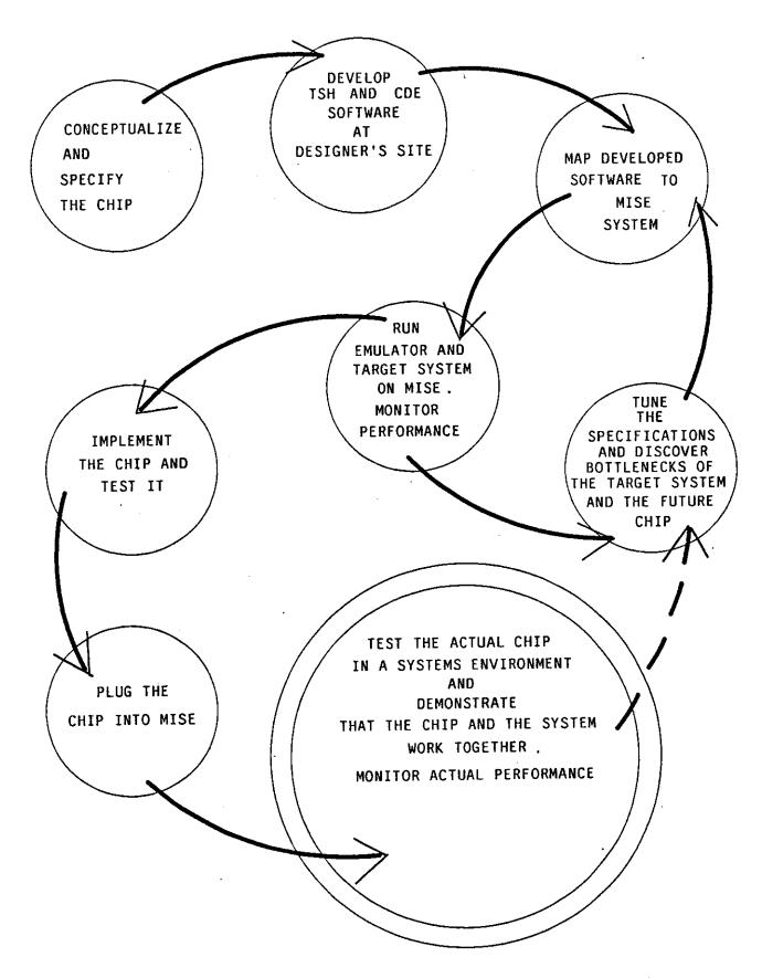
Figure 3: System Design Process Involving MISE.
