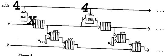
Figure 8. Another two-level pipelined systolic array for two or high dimensional convolutions er
