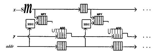
Figure 6. Systolic array using adaptive weights for interpolation and resampling
