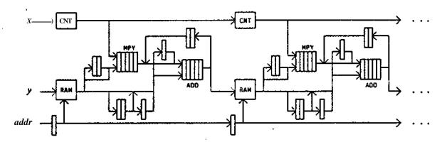
Figure 14. Two consecutive cells in the two-level pipelined systolic array for the FFT
