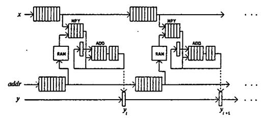
Figure 12. Two-level pipelined systolic arrayfor complex matrix multiplication
