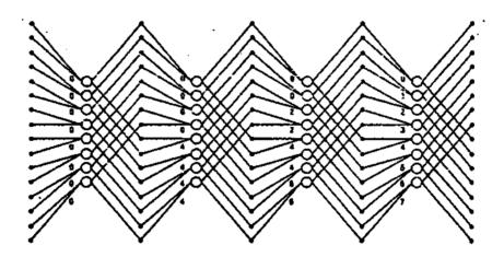
Figure 13. Constant geometry version of the FFT algorithm
