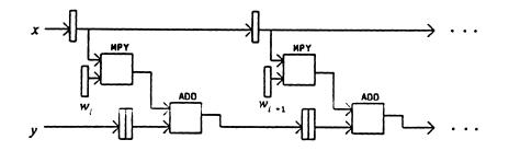
Figure 4. Cell structure for the I-D convolution array of Figure 3
